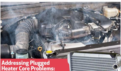
Today's vehicles are manufactured with very tight heater cores that can become plugged overtime. It is not uncommon for a 4-year-old vehicle, if the coolant system is not flushed annually and recharged with new coolant, will simply plug-up. #1 symptom is no heat.
